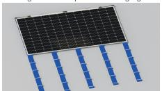
Gluing at the ribs of the CS support, installing and flattening the assembly, placing the junction box side at the service walkway, and rolling the surface of the module with a plastic roller to ensure a good bond between the module and the CS supports.
